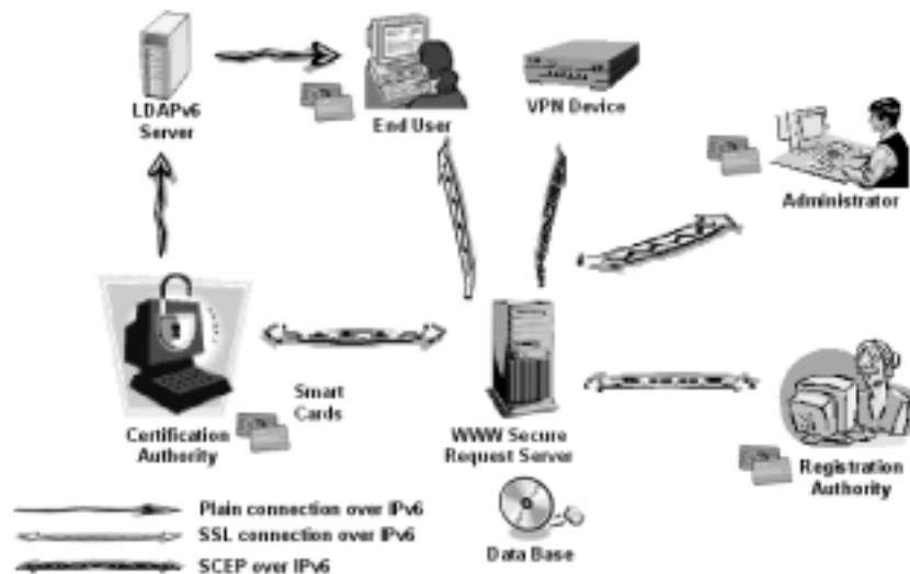
Figure 1: Java IPv6 PKI Architecture and Communications
